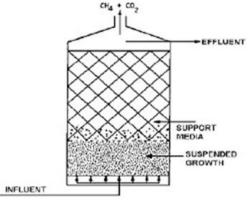
Figure 1. Anaerobic Filter
